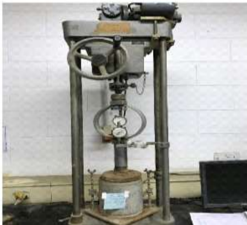
Figure 7: CBR test assembly
