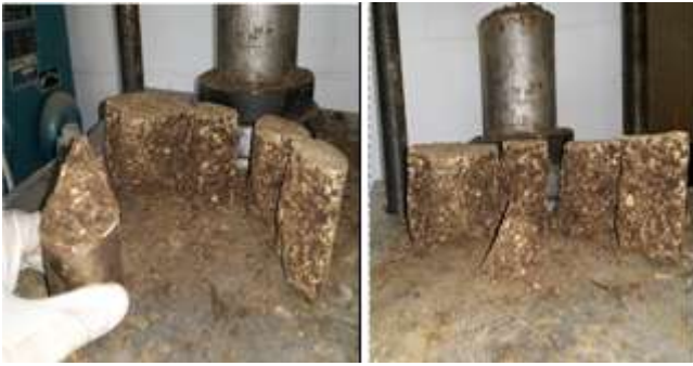
Figure 6: The failure mode at fluid content equal to 16%
