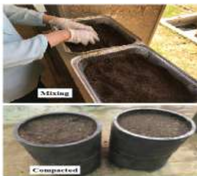
Figure 3: Preparation of asphalt stabilized specimen
