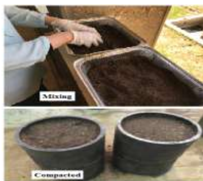
Figure 3: Preparation of asphalt stabilized specimen
