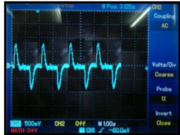
Figure 4: Practical EOG signals at the amplifier output (the signal goes negative peak for left movement of the eyes, while the signal goes positive peak for right movement of the eyes).
