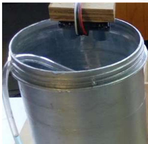
Figure 6: Location and physical assembly of the ultrasonic sensor in the structure.
