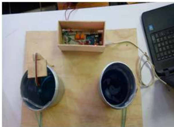
Figure 7: Final assembly of the structure with the ultrasonic sensor and Arduino UNO.
