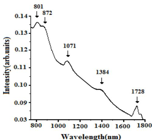
**Figure 3:** NIR absorption spectrum of Dy<sup>3+</sup> ions doped NaCaAlPO<sub>4</sub>F<sub>3</sub> phosphor.
