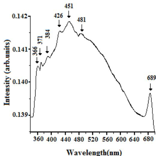
**Figure 2:** UV-Vis absorption spectrum of Dy<sup>3+</sup> ions doped NaCaAlPO<sub>4</sub>F<sub>3</sub> phosphor
