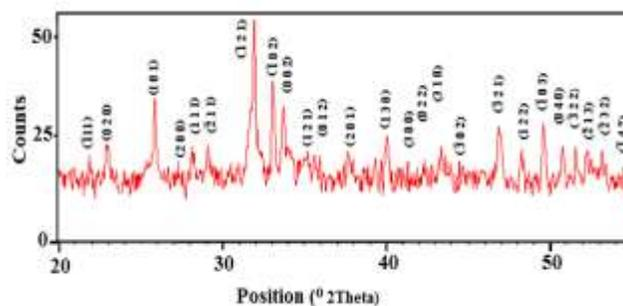
**Figure 1:** Powder X-ray diffraction pattern of Dy<sup>3+</sup> ions doped NaCaAlPO<sub>4</sub>F<sub>3</sub> phosphor.
