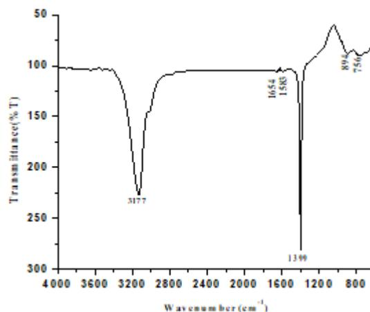
**Figure 6:** FT-IR spectrum of Dy<sup>3+</sup> ions doped NaCaAlPO<sub>4</sub>F<sub>3</sub> phosphor
