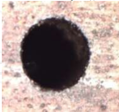
Figure 8: Top view of drilled hole using stereo microscope
