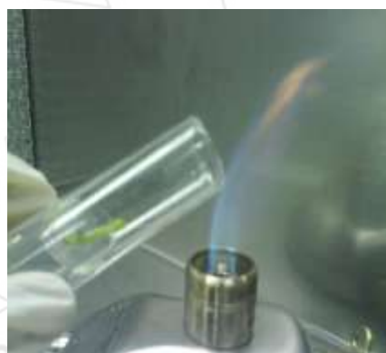
Figure 16: Vial mouth flamed as part of aseptic manipulation
