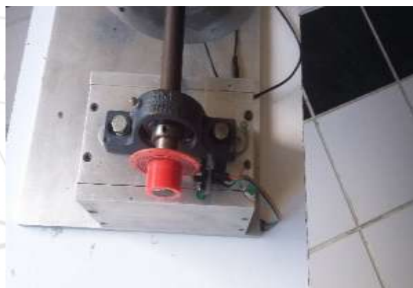
Figure 14: Positioning of the optical barrier sensor
