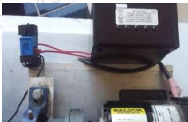
Figure 15: Position of the current sensor.
