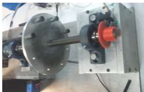
Figure 12: Disc with unbalanced load.
