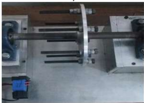
Figure 11: Disc with balanced load
