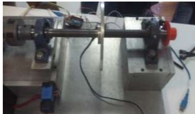
Figure 13: Stability disc and arrow of the rotodynamic system
