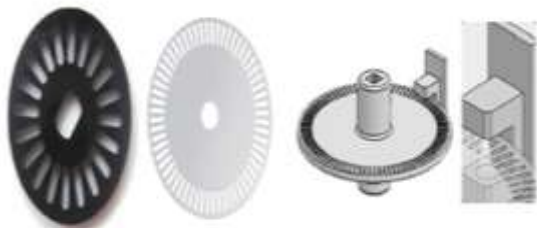
Figure 7: Disk with slots (encoder).
