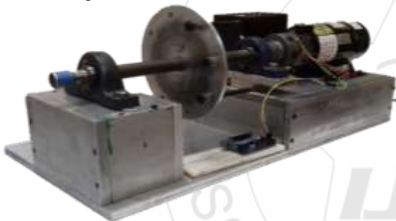
Figure 13: Testing bench with unbalanced load
