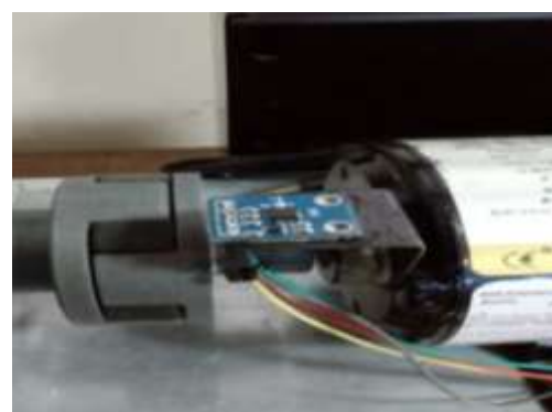
Figure 6: Accelerometer in the testing bench
