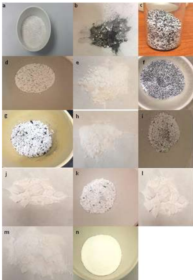
Figure 1: Chicken eggshell powder before and (a) before calcination (b) 700°C for 1-2h (c) 700°C for 3h (d) 700°C for 4h (e) 700°C for 5h (f) 750°C for 1-2h (g) 750°C for 3-4h (h) 750°C for 5h (i) 800°C for 1-2h (j) 800°C for 3-5h (k)
