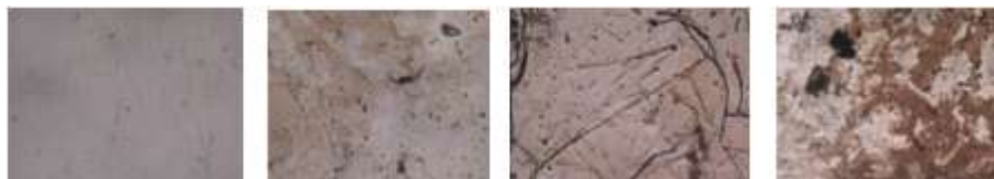
Figure 7: Micrograph of pure LAP and irradiated single crystals (a: pure, b: 1 \times 10^{16} c: 5 \times 10^{16} , d: 1 \times 10^{17} )
