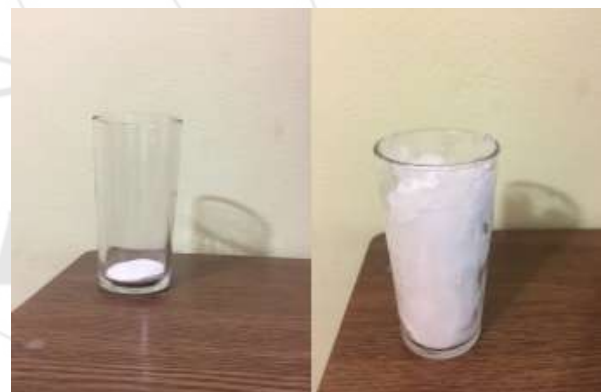
Figure 1: Dry (SAP) in the left cup. The right cup after adding some water
