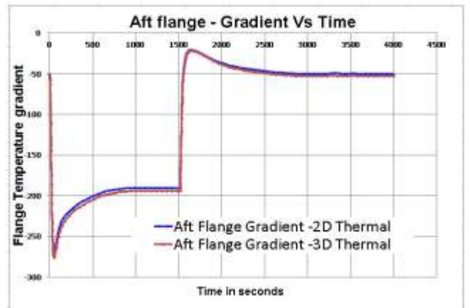
Figure 12: Aft Flange Temperature Gradient
