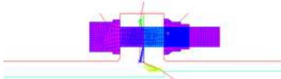
**Figure 3:** Convection and Fluid Elements (2D)
