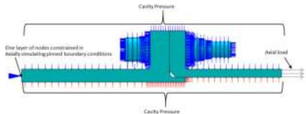
Figure 8: Structural Model Loads
