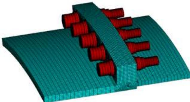
**Figure 2:** Bolted Flange – 3D Mesh Model (Thermal & Structural)
