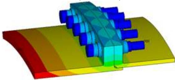
Figure 10b: 3D Temperature Contour At Max Gradient Time Point (47 Seconds)
