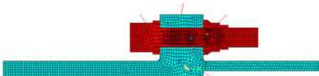
**Figure 1:** Bolted Flange – 2D FE Model (Thermal)
