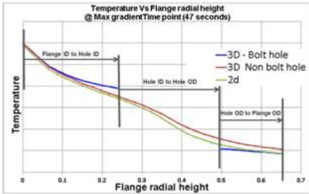
**Figure 13:** Forward Flange, ID to OD Temperature Profile
