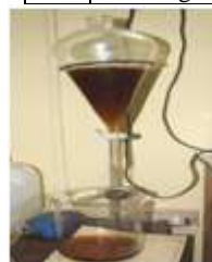
Figure 1: Filtering of raw WCOBD
