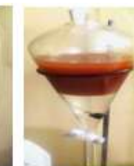
Figure 5: Methyl ester and water separation
