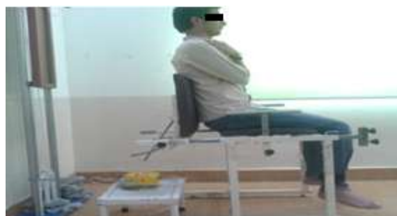
Figure 3: Measurement of knee extensor strength
