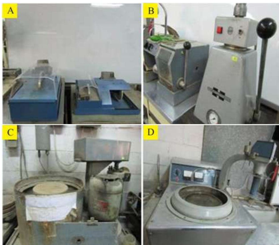
Figure 3: Cutting, grinding, polishing devices used in this study, (A: cutting machine), (B: mounting preparation device), (C: grinding machine), (D: polishing and buffing machine)
