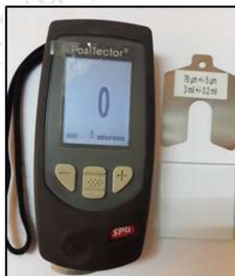
Figure 4: PosiTector device with standard plate and glass for the device normalization used for measuring the surface roughness.
