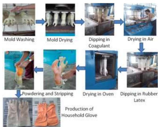
Figure 2: Flow Diagram of the Production of Household Glove
