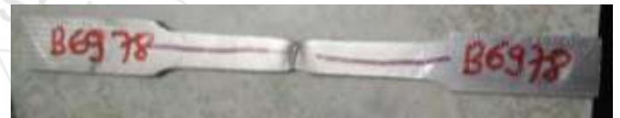
Figure 6: Fractured aluminum specimen
