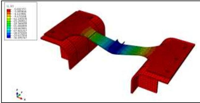
**Figure 14:** F.E simulation of fracture test
