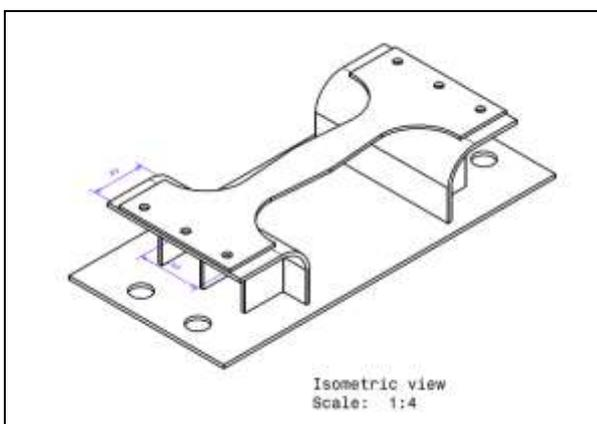
**Figure 10:** Mixed mode fracture test set-up
