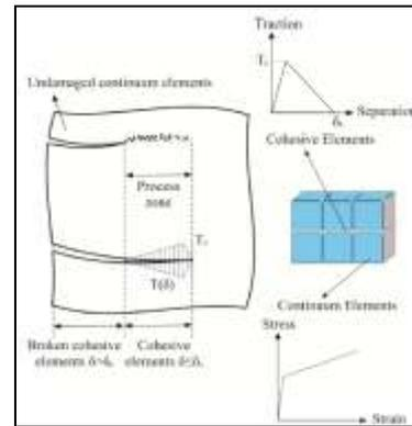
**Figure 1:** Process zone in cohesive crack model [4]
