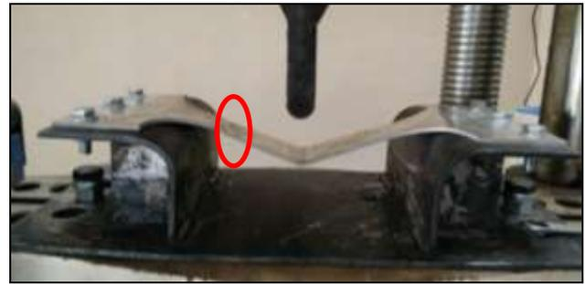
**Figure 11:** Mixed mode fracture test.
