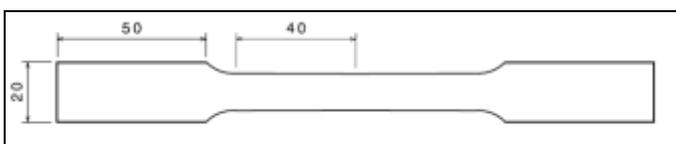
Figure 4: Tensile test specimen (All dimensions in mm)
