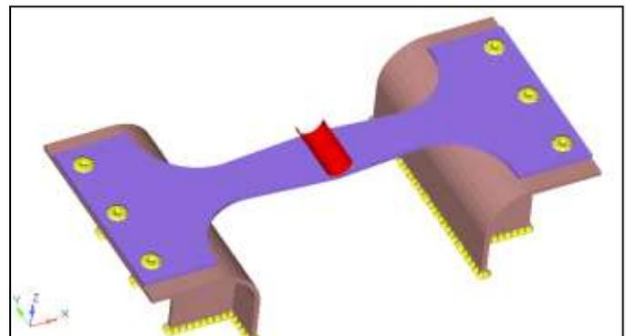
**Figure 12:** F.E test set up of fracture test.
