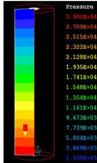
Figure 2: Pressure variation in the fluid along the cylinder height (1000 s, P=500 MPa)
