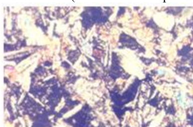
Photo 2. Dolerite with Ophitic texture showing Labrodorite laths in Augite crystals.
