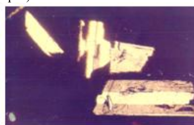
Photo 3. Vitrophyric Basalt showing Labrodorite laths embedded in glassy ground mass.
