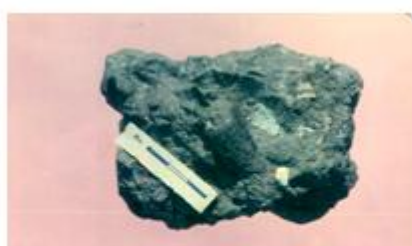
Photo 4. Hand specimen photograph of volcanoclastic Breccia with angular pebbles of ultrabasic and basic rocks.
