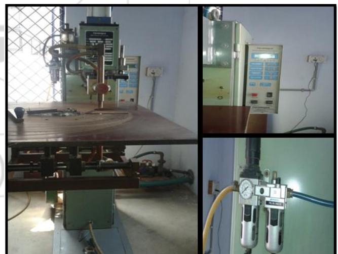
Figure 1: General setup of Resistance Spot Welding Process
