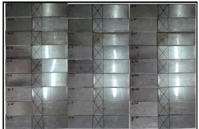
Figure 3: Specimens of Spot welded for SS304
