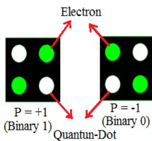
**Figure 1:** QCA cell and two possible polarizations
