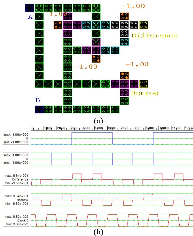
**Figure 8:** (a) QCA layout Half-Subtractor (b)Simulation results
