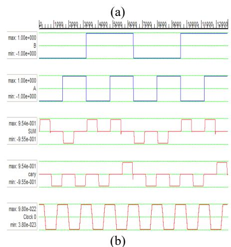
**Figure 8:** (a) QCA layout Half-Adder (b)Simulation results
