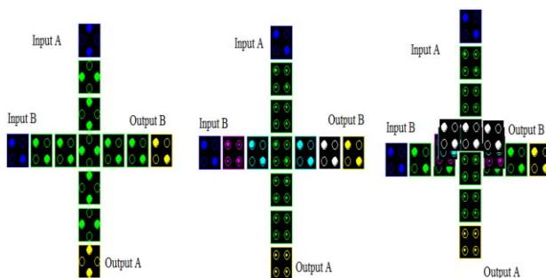
**Figure 5:** Wire crossing methods: (a) Single layer wire crossing (b) Logical crossing (c) Multi-layer wire crossing
