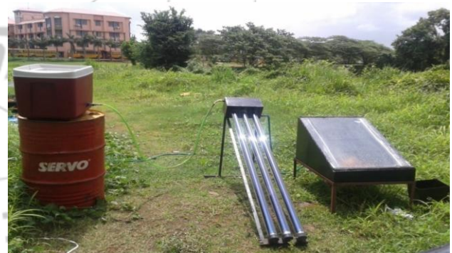
Figure 1: Experimental Setup of Still with Evacuated Tube Collector
