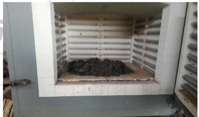
Figure 1: Esklo s.r.o heating kiln –Sample in position
