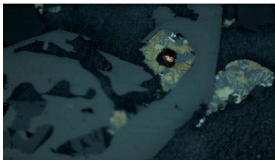
Figure 1: Complex sulphide splice - "copper-bearing pyrite globule": in the center of pyrite grains is metallic copper bead size of 3 microns. Pyrite grains bordered magnetite "ribbon"
