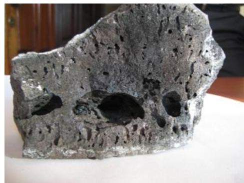
Figure 2: Lump of whole copper ore size 100 mm*70mm*42mm
