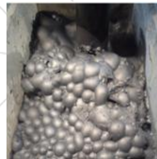
Figure 7: The floating froth underspoil water
