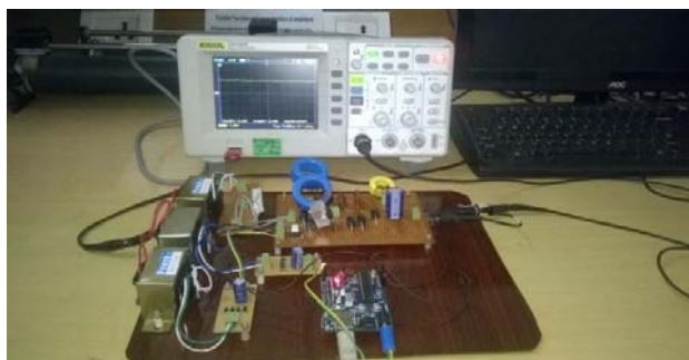
Figure 4.7: Hardware implementation of Bridgeless Cuk PFC rectifier with positive output voltage made
