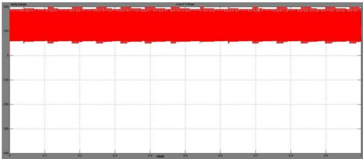
Figure 19: Output voltage waveform for conventional transformer less dc-dc converter
