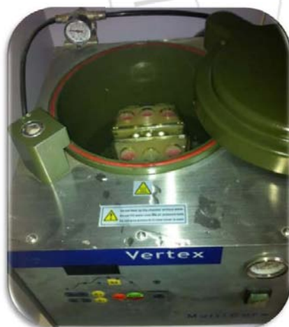
Figure 3: The flask was placed in the pressure vessel
