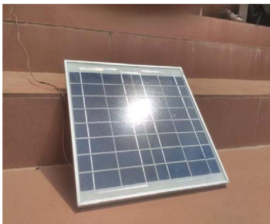
Figure 6.1: Solar panel of 60W
