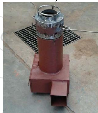
Plate 3.1: Gasifier stove under fabrication
