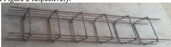
Figure 1: Reinforcement for control beams
