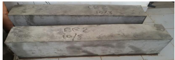
Figure 2: Control beams after casting
