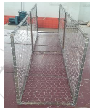
Figure 3: Skeletal reinforcement covered with chicken mesh
