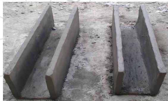
Figure 4: Ferrocement formwork after casting
