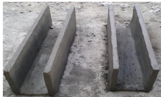
Figure 4: Ferroceement formwork after casting
