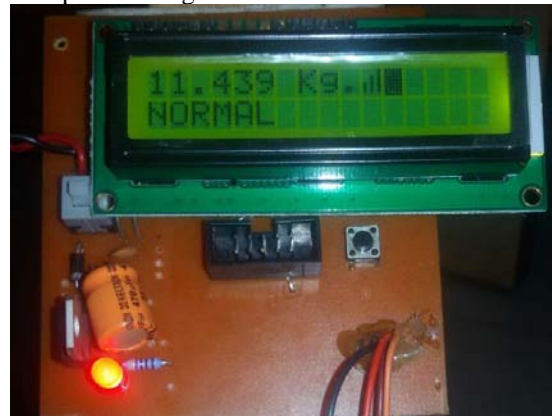
Figure 10: Normal Stage Threshold Pressure > 10KG and < 20 KG
