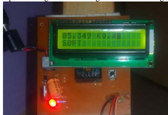
Figure - 9: Soft Stage Threshold Pressure > 2KG and <= 20 KG
