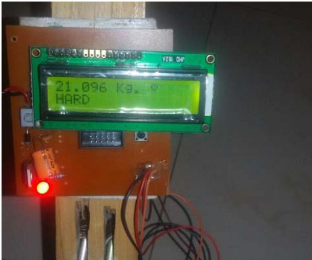
Figure - 11: Hard Stage Threshold Pressure > 20 KG
