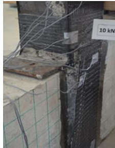
Figure 10: U-shape cut by the belt's edge stress of C1S1
