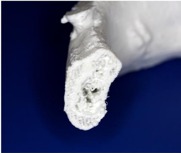
Figure 1: Transversal cross-section of 3D-printed simulation model imitating the typical corticocancellous bone structure.
