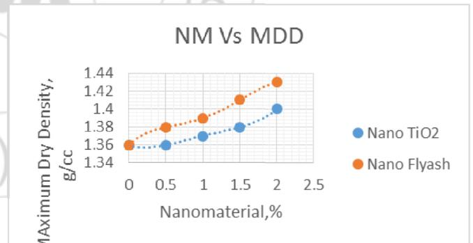
**Figure 4:** Maximum Dry Density for different nanomaterials
