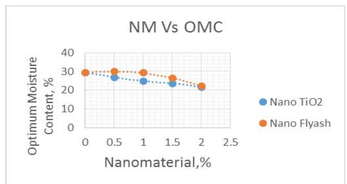
**Figure 5:** Optimum Moisture Content for different nanomaterials
