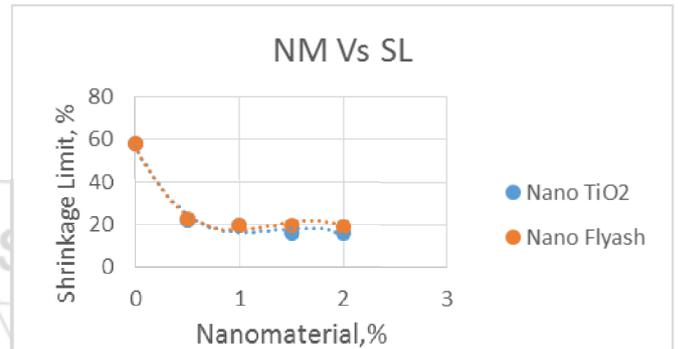
**Figure 3:** Shrinkage Limit for different nanomaterials
