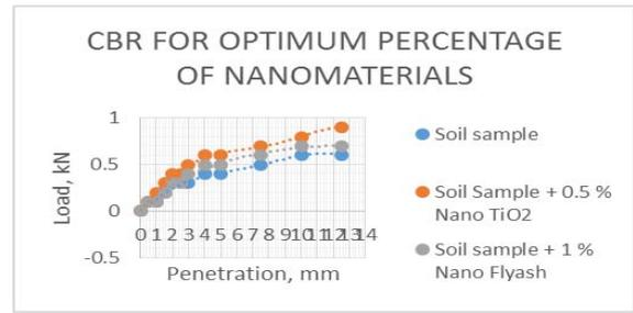
**Figure 6:** Load vs Penetration curve for CBR test
