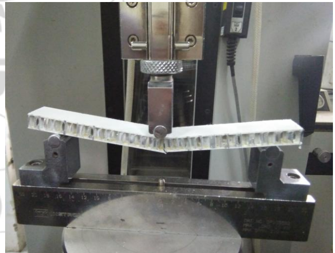
Figure 2: Experimental setup for three point bending
