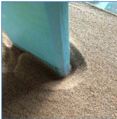
Figure 5: Scour hole geometry around chamfered pier (Run 15)
