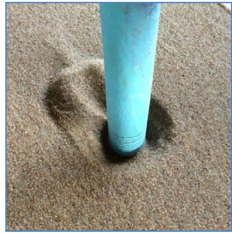
Figure 6: Scour hole geometry around circular pier (Run 21)
