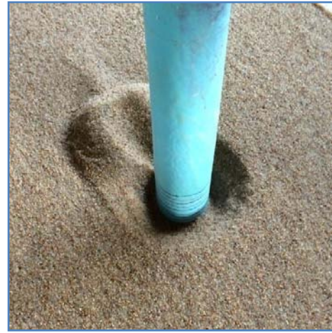
Figure 6: Scour hole geometry around circular pier (Run 21)
