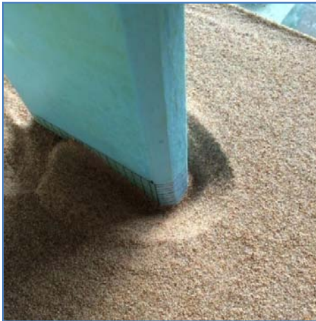
Figure 5: Scour hole geometry around chamfered pier (Run 15)
