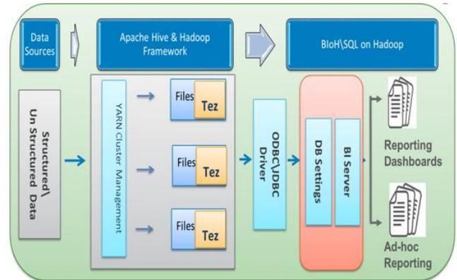
**Figure 6:** Access on Apache Tez (High Level Architecture)
