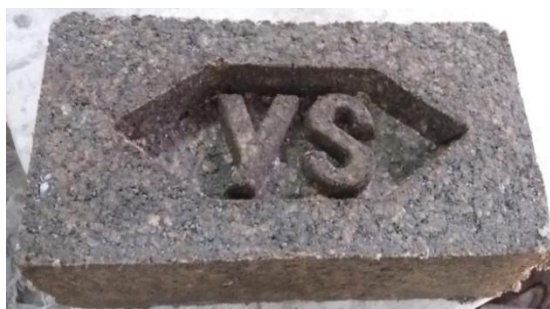
Figure 2.3.1: Papercrete bricks after casting
