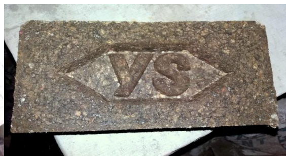
Figure 2.3.1: Papercrete bricks after casting
