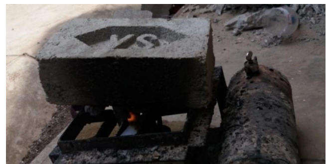
Figure 3.8.1: Fire test of papercrete brick
