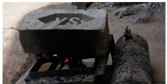
Figure 3.8.1: Fire test of papercrete brick
