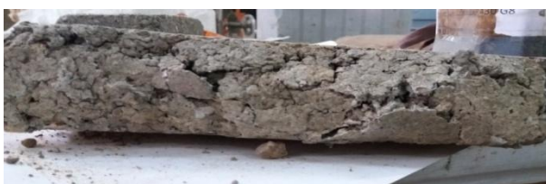
Figure 3.1.1: Brick after testing
