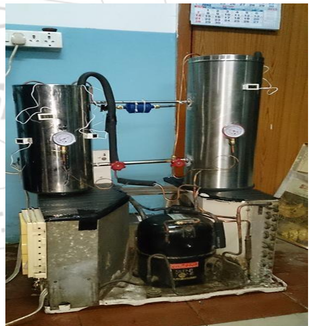
Figure 1.4: Air conditioning cum Water Dispenser System
