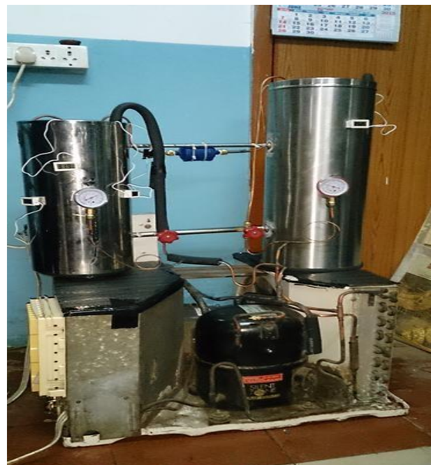
Figure 1.4: Air conditioning cum Water Dispenser System
