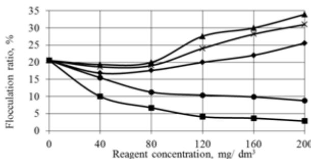
Fig. 4. Effect of reagent concentration on the flocculation ratio of the particles of iron-vanadium
