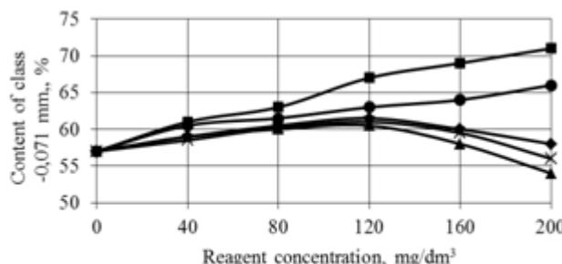
Fig. 3. Effect of reagent concentration on the content of class -0.071 mm in iron-vanadium middlings:
