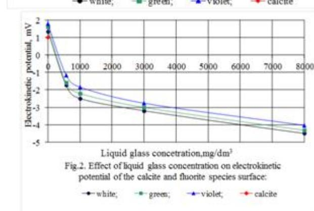
Fig.2. Effect of liquid glass concentration on electrokinetic potential of the calcite and fluorite species surface:
