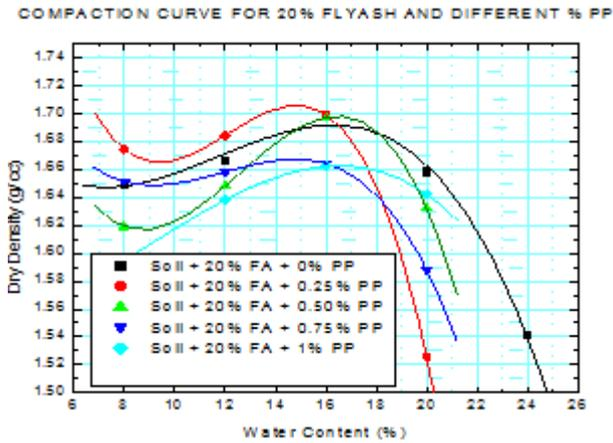
**Figure 1:** Compaction curve for different PP fibres content
