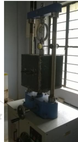
Figure 3: Vertical loading on Micropile
