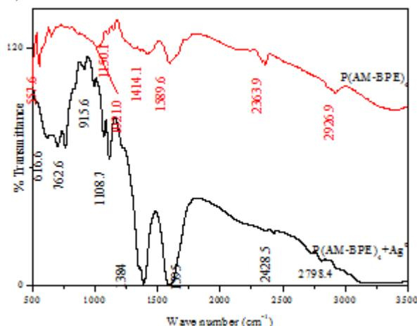
**Figure 1:** FTIR spectra of pure P(AM-BPE)<sub>4</sub> hydrogel and P(AM-BPE)<sub>4</sub>+Ag<sup>0</sup> nanocomposite hydrogel
