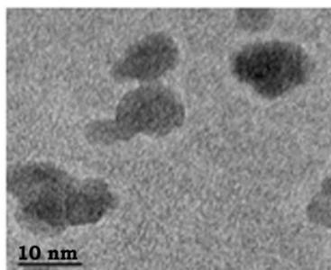
Figure 6: TEM images of P(AM-BPE)<sub>4</sub>+Ag<sup>0</sup> nanocomposite hydrogel
