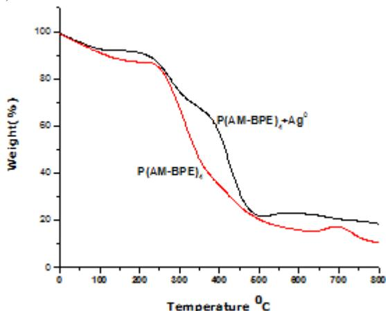
**Figure 3:** Thermogravimetric analysis of P(AM-BPE)<sub>4</sub> hydrogel and P(AM-BPE)<sub>4</sub> +Ag<sup>0</sup> nanocomposite hydrogel
