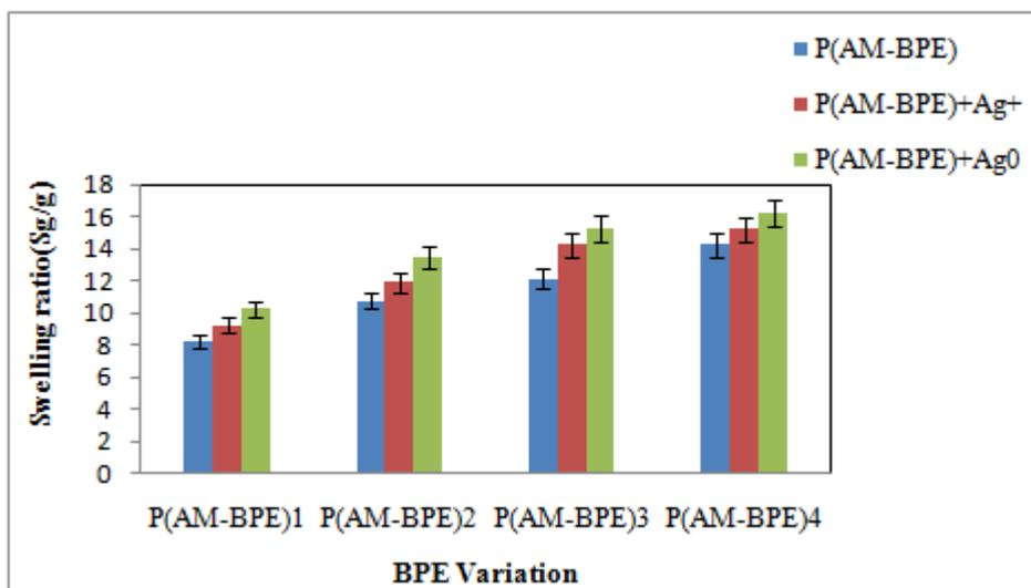
Figure 7: Swelling behaviour of P(AM-BPE), P(AM-BPE)+Ag<sup>+</sup> varied hydrogels and Ag<sup>0</sup> nanocomposite
