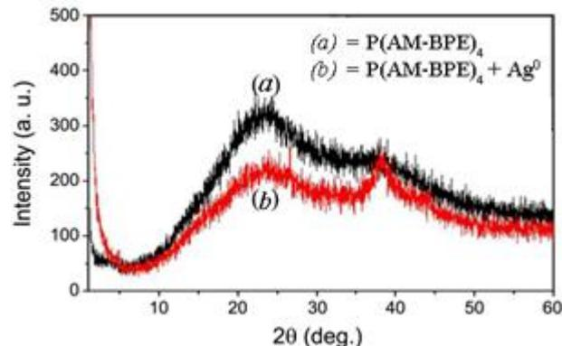
**Figure 4:** XRD patterns of pure P(AM-BPE)<sub>4</sub> hydrogel and P(AM-BPE)<sub>4</sub>+Ag<sup>0</sup> nanocomposite hydrogel
