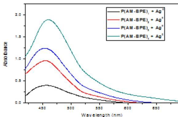
**Figure 2:** UV-vis of spectra of P(AM-BPE)<sub>4</sub>+Ag<sup>0</sup> nanocomposite hydrogels
