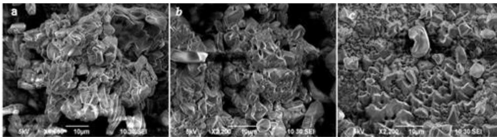
Figure 5: SEM images of: pure P(AM-BPE)<sub>4</sub>, P(AM-BPE)<sub>4</sub>+Ag<sup>+</sup> and P(AM-BPE)<sub>4</sub>+Ag<sup>0</sup> nanocomposite hydrogels
