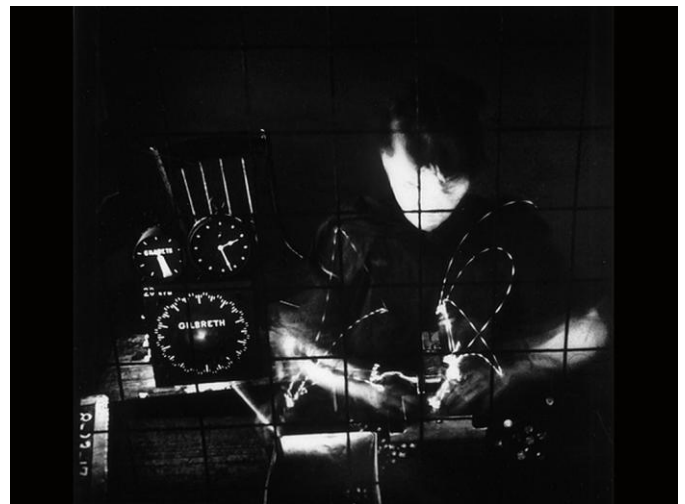
Figure 11: Chrono Cycle Graph Of An Operator Performing Diamond Variations
