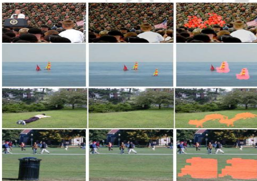
Figure 6: Each row indicates different images: first column is the original image; second column is the tampered image and the third column is the detection result of the algorithm.
