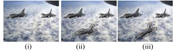
Figure 7: CRM manipulation and its detection result. (i) Original image with two aircrafts (ii) forged image with three aircrafts by copy-move forgery (iii) forged image showing three aircrafts by copy-rotate-move (CRM) forgery.
