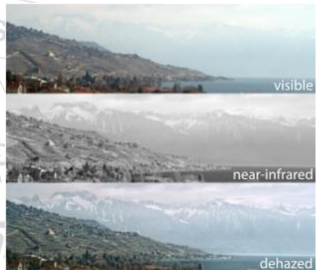
Figure 7: Example of a scene containing haze. Note the higher contrast and sharpness in the near-infrared image and the de-hazed image using our method compared to the visible image.
