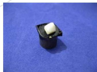
Figure 2: The specimens were glued to copper stubs.
