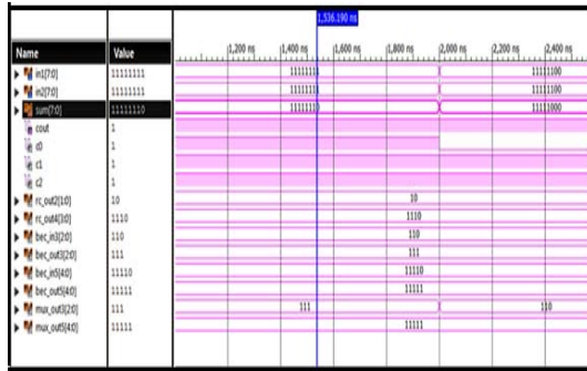
Figure 6: Simulation result for carry select adder FCU1
