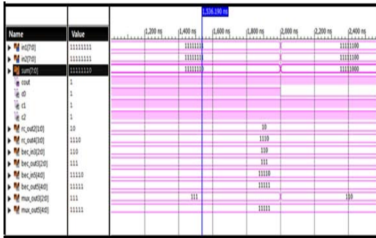
Figure 6: Simulation result for carry select adder FCU1
