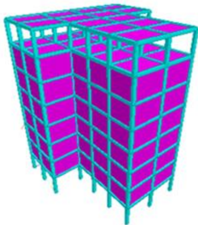
Figure 7: Three dimensional view of G+6 Building with top floor as soft storey
