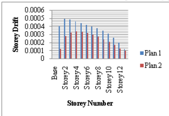
Figure 13: Storey Drift of G+12 Buildings
